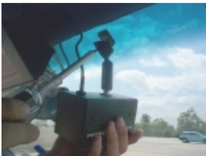
View of camera being attached to windshield mount. Note: Cable of camera goes upwards into headliner.
