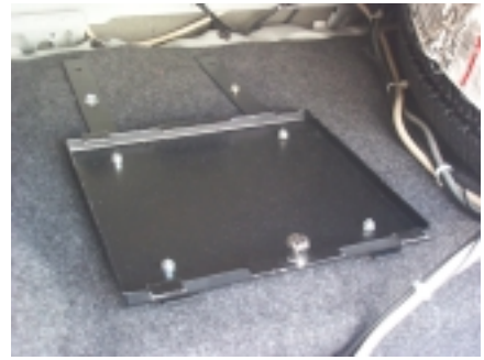
Completed assembly of brackets and base plate of vault
