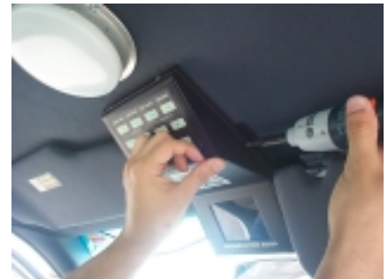
View of control console being mounted with wires already attached to connections
