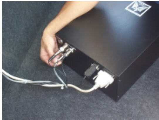
Attaching the cables to the rear of the vault.
