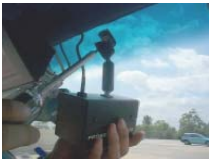
View of camera being attached to windshield mount. Note: cable of camera goes upwards into headliner.
